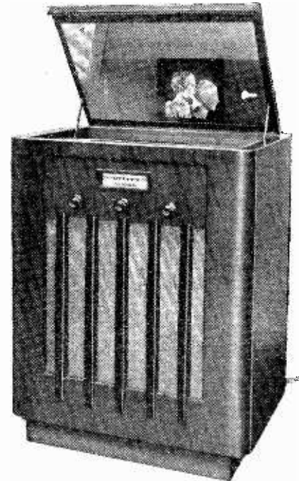
The Telefunken home-television receiver in which the picture is viewed through a mirror. It also provides sound reception.
